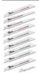
8% Cobalt Metal Reciprocating Saw Blades. These extra-tough Bi-Metal professional quality blades are used for metal, plastics, fiberglass, and plaster. The 8% cobalt Matrix II cutting edge is electron-beam welded to a high strength steel backer, for greater wear resistance and longer life, and to give you the sharpest, fastest cuts.
